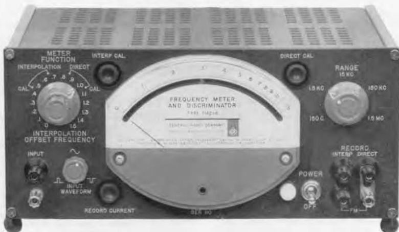
Figure 1. Panel View of the Type 1142-A Frequency Meter and Discriminator. The instrument is housed in a rack-bench cabinet (see "The Case of the Well-Designed Instrument," General Radio Experimenter , March, 1960, page 7).
